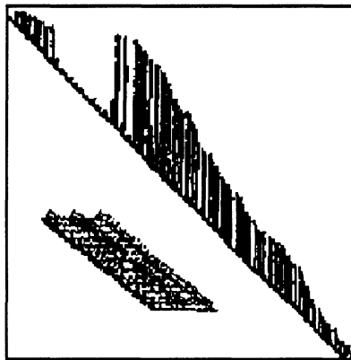
Figure 4.7 Skyline storage scheme for stiffness matrix before and after decomposition
